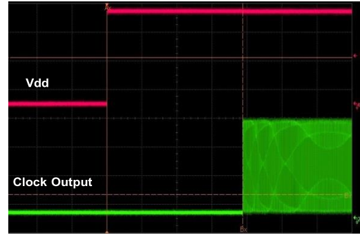
Figure 17. Startup Waveform vs. Vdd
