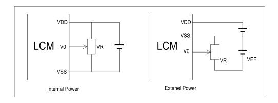
$V_{DD^{\sim}}V_0$ : LCD Driving voltage
