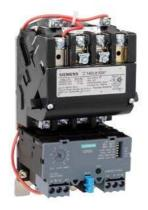
Non-reversing motor starter Size 1 Single phase full voltage Solid-state overload relay OLRelay amp range 3-12A 110-120/220-240VAC 60HZ coil Combination type No enclosure
