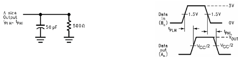
FIGURE 3. B to A Direction Test Load and Waveforms for Outputs A 1 - A 4
