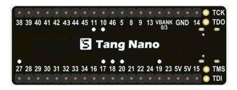
Note: The digital number is the chip pin number, and the dot identified by the dot is the GCLK pin.
