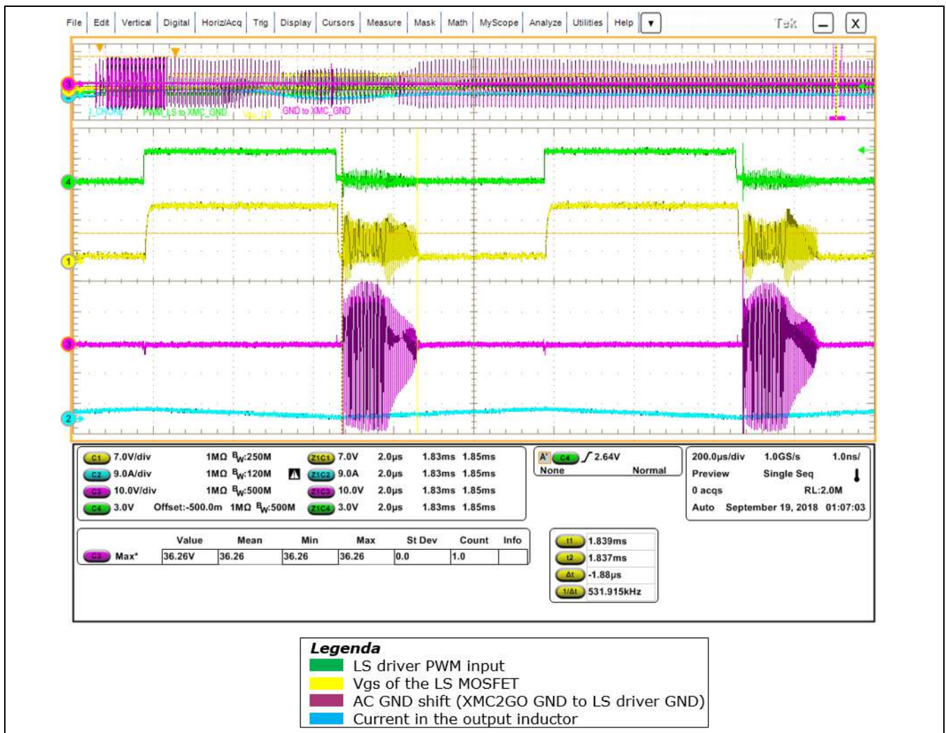
Figure 9 Destructive shoot-through event in the TDI HB BC evaluation board with standard single-channel LS driver, in the worst configuration of GND inductance and with 18 Ω load
