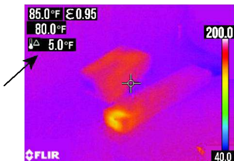
Fig. 8-4 Type-K / IGM Temperature Differential Reading Example
