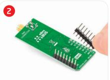
Turn the board upside down so that bottom side is facing you upwards. Place shorter parts of the header pins in both soldering pad locations.
