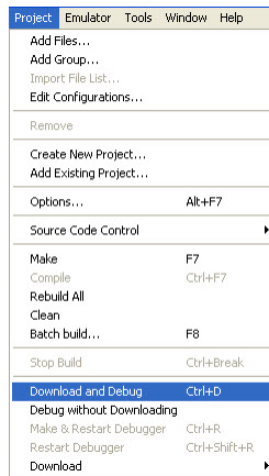
Figure 15. Downloading and debugging the RF Breakout Module project
