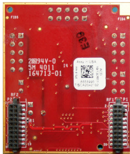
Figure 3. Back side of the RF Breakout Module, showing the RF connectors
