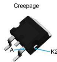
Figure 13. Creepage without top coating
