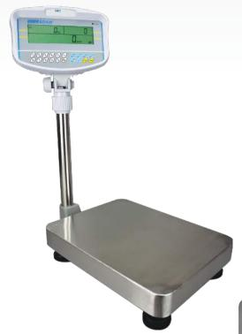
The GBC is a fully featured counting scale with numeric keypad for unit weight and sample entry. The large, brightly backlit display shows unit weight, total weight and number of pieces. With a grade 304 stainless steel pan and pillar-mounted ABS plastic indicator, the GBC provides a durable, reliable solution for industrial counting tasks. Power is supplied by a mains power cord or the built-in, rechargeable battery.
