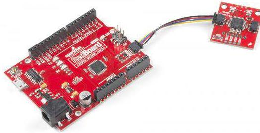
If, however, you are using an older SparkFun RedBoard, you'll need an assembled Qwiic Shield, so if you haven't done that yet, now would be the time to head on over to that tutorial.
