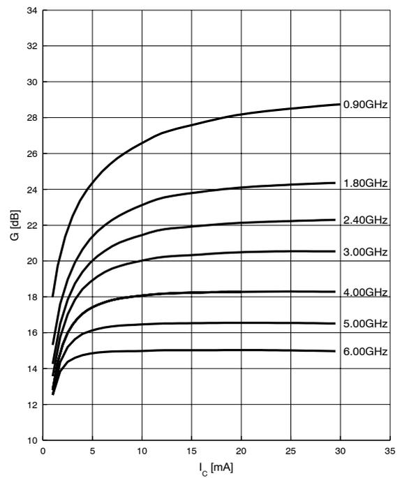
**Power gain  $G_{ma}$ ,  $G_{ms} = f(V_{CE})$**
