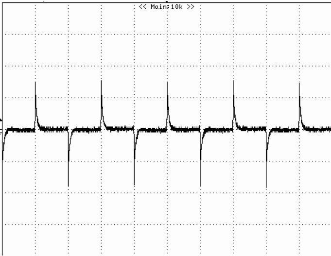
Figure 17: Typical transient response to step load change at 1A/\mu S from 100%~ 50%~100% of I_o , max at 12V_{in} , 5.0V_{out} ( C_{out} = 1\mu F ceramic, 47\mu F+10\mu F ceramic) CH1 : VOUT, 0.1V/div, 5mS/div
