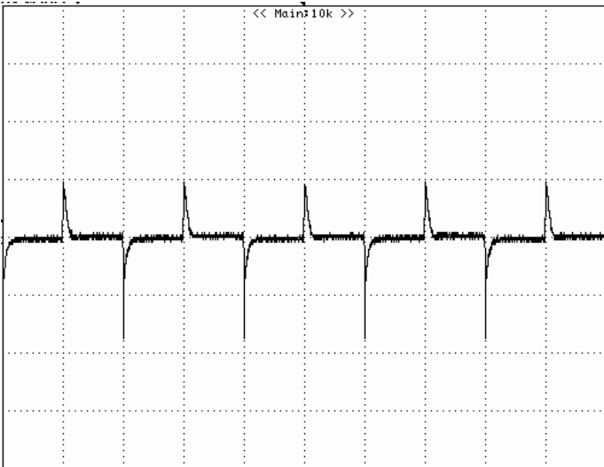
Figure 19: Typical transient response to step load change at 1A/\mu S from 100%~ 50%~100% of I_o , max at 12V_{in} , 1.2V_{out} ( C_{out} = 1\mu F ceramic, 47\mu F+10\mu F ceramic) CH1 : VOUT, 0.1V/div, 5mS/div
