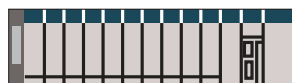
Five Analog Output Units of 8 points each Five Analog Input Units of 8 points each
