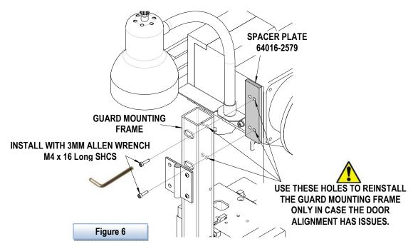
Important Locate the new spacer plate (64016-2579) <u>BETWEEN</u> the guard mounting frame and the press. **Note:** Make sure to use the <u>RIGHT SIDE</u> set of mounting holes. See Figure 6.
