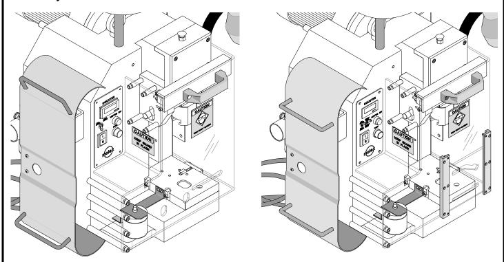
Starting in 2012 all new presses will have the 64016-2595 factory installed. For existing presses, the 64016-2595 safety guard upgrade kit can be purchased separately.
