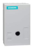
Electrically held lighting contactor, Contactor amp rating 20A, 0 N.C. / 4 N.O. Poles, 347VAC 60HZ coil, Non-combination type, (no disconnect device), Enclosure NEMA type 1, Indoor general purpose use
