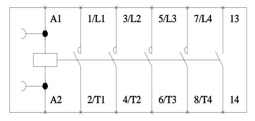
LEN00B004 Wiring Diagram
