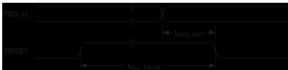
Figure 6. RESET and Profile Select Timing
