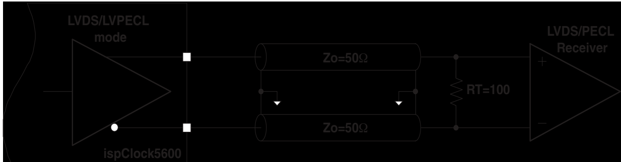
Figure 22. Configuration for LVDS and LVPECL Output Modes
