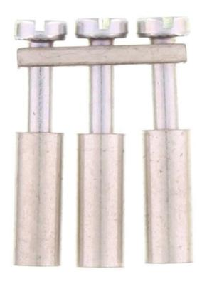
Cross-connector, No. of poles: 3, Mounting type: Can be screwed on, Width: 17 mm, Rated cross-section: 4 mm², Colour: natural
