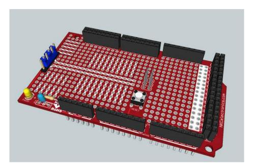
The kit includes the board and many extra components. What you finally end up installing on the ProtoShield will be based on your requirements. But in general, I recommend soldering all the female headers, as they are needed to bring all the signals and POWER from the chipKIT Max32 board to the ProtoShield.
