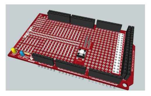
The little 6-pin male header with the 2 jumpers are used to configure how you want to use the 2 power BUSES in the middle of the board. You can send +5V to one of them, GND to the other, or +5 or GND to both of them at the same time.
