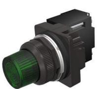
30mm BlackMax, Epoxy Coated Corrosion Resistant Complete Metal Unit Illuminated Indicator Light Transformer type, 600V AC Super Bright LED Lamp, BA9s Glass Lens, Green UL Listed, CSA Certified NEMA 1,3,3R,4,4X,12,13 & Automotive Standards
