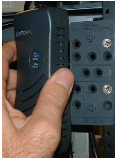
2. Attach the Spider to the bracket's mounting posts
