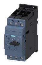
Circuit breaker size S2 for motor protection, CLASS 10 A-release 14...20 A N-release 260 A screw terminal Standard switching capacity
