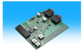
The EZURiO Winbond Codec Evaluation Board plugs into the EZURiO Developers kit and allows you to rapidly test and evaluate *Bluetooth* audio applications using the EZURiO *Bluetooth* Intelligent Serial Module to implement the wireless link.
