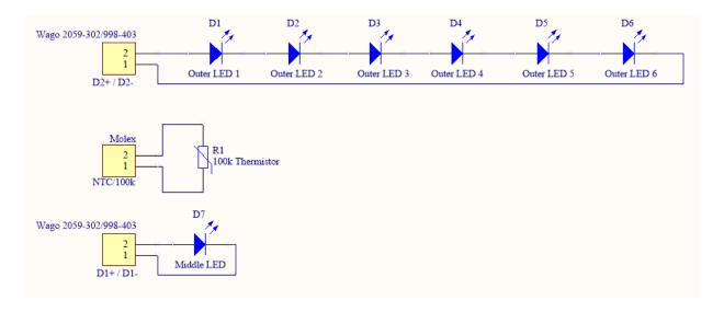
Sevengine LEDs of the same type can be connected in series. The following figure shows an example of how several Sevengines are connected in series.
