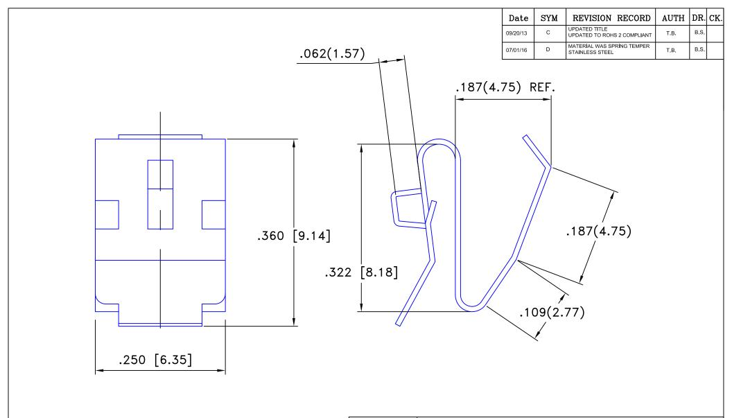
MATERIAL: 0.010" SPRING STEEL, NICKEL PLATED ROHS 2 COMPLIANT
