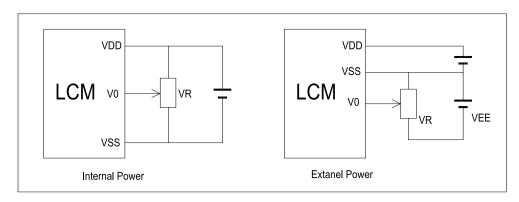
$V_{DD^{\sim}}V_0$ : LCD Driving voltage
