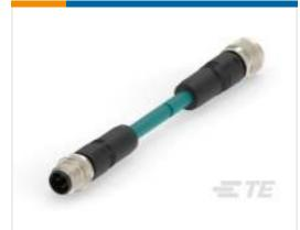
TE Part # CAT-SI113-M1C M12 D-code 4pin Male to Female Cable Assembly, Cat5e TPE 24AWG Unshielded
