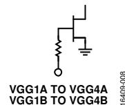
Figure 8. VGG1A to VGG4A and VGG1B to VGG4B Interface Schematic
