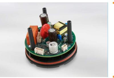
LUMAWISE ENDURANCE N ENHANCED BASE DE-RISKS PROJECT SCHEDULES AND COST OF DESIGN CHANGES OF NEMA/ANSI STREET AND OUTDOOR LIGHTING CONTROL SOLUTIONS. THE ENHANCED BASE TAKES OUR LIGHTING CONTROL BASE ASSEMBLY TO THE NEXT LEVEL OF PERFORMANCE BY PROVIDING AC POWER SWITCHING AND DC POWER SUPPLIES
