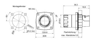
Main Dimensions Extension \*for max. wire cross-section pay attention to the cross-section of used contacts
