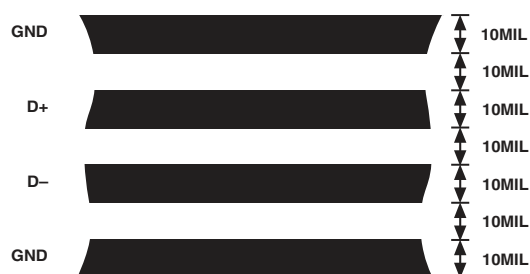
Figure 6. Arrangement of Signal Tracks
