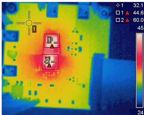
Figure 18: Thermal Image at V_{IN} = 12V , I_{OUT} = 6A (IR3863: 60°C, Inductor: 45°C, PCB: 32°C)
