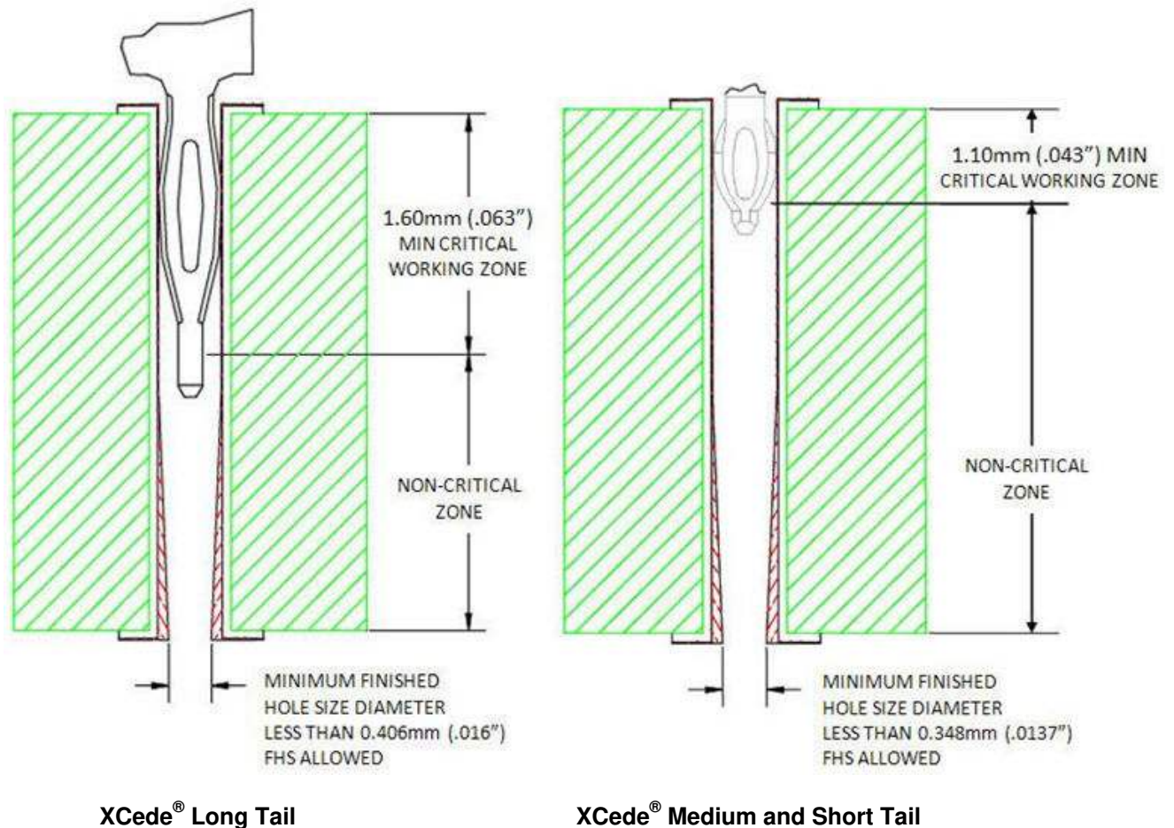
Figure 11: XCede® Compliant Pin Critical Zones
