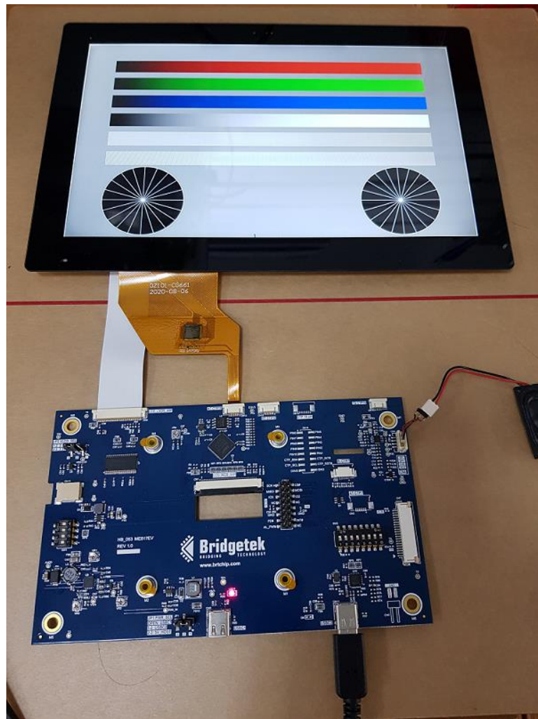
Figure 5-4 - PC setup with 10.1" 1280x800 panel
