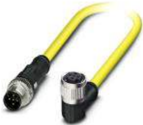
Sensor/Actuator cable, 5-position, TPE, Plug straight M12 SPEEDCON, A-coded, on Socket angled M12 SPEEDCON, A-coded, Cable length: 5 m
