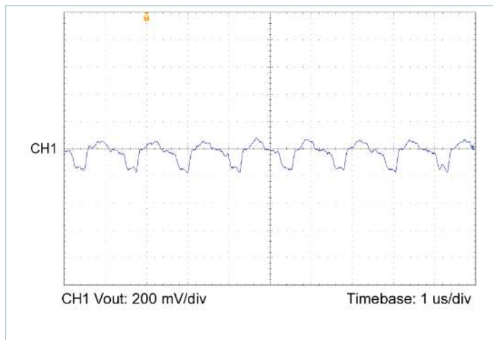
Figure 18 — Output voltage ripple, V_{IN} = 43\text{V} , V_{OUT} = 24.0\text{V} , C_{OUT\_EXT} = 470\mu\text{F} , R_{LOAD} = 5.714\Omega
