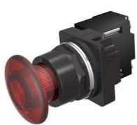
30mm BlackMax, Epoxy Coated Corrosion Resistant Complete Metal Unit Illuminated Push-Pull Operator Full Voltage, 24V AC/DC Incandescent Lamp Mushroom Head Cap Small 1 3/4" (44.5 mm) Plastic, Red 3 Position Pull-Momentary/Push-Maintained UL Listed, CSA Certified NEMA 1,3,3R,4,4X,12,13 & Automotive Standards
