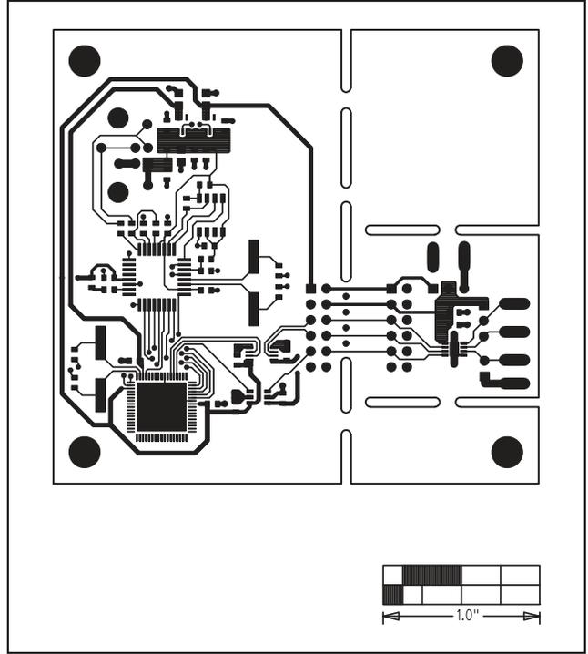
Figure 6. MAX5422 EV Kit PCB Layout—Component Side
