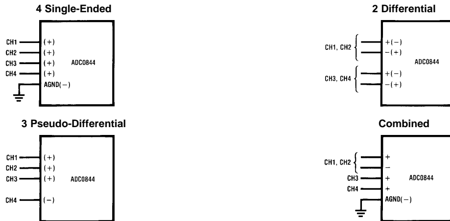
Figure 12. Analog Input Multiplexer Options
