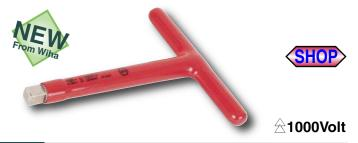
290 12 Insulated 1/2" Drive T-handle, With Insulated Handle Insulation according to EN/IEC 60900 specification, up to 1000 Volt. Individually Tested. Blade chrome-vanadium steel, hardened.
