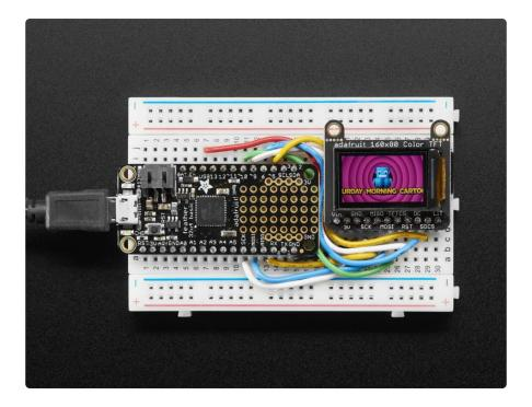
It's the size of your thumbnail, with glorious 160x80 pixel color... it's the Adafruit Mini TFT Breakout! This very very small display is only 0.96" diagonal, packed with RGB pixels, for making very small high-density displays.
