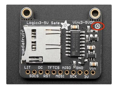
On the reverse side of the TFT, the Revision B version has a smaller chip on the back. The display is plugged in on this revision and it has a B inside of a circle in the top center:
