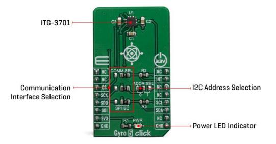
Typically, higher dps range results in lower sensitivity. Therefore, the ITG-3701 allows to dynamically select the full-scale range (FSR) value in several discrete steps:  $\pm$ 500,  $\pm$ 1000,  $\pm$ 2000 and  $\pm$ 2000 dps. This allows optimized performance for a given usage scenario. For example, if used in applications with faster angle rates such as sports equipment monitoring (golf club or tennis racket), a higher FSR might be required, at a cost of lower sensitivity.
