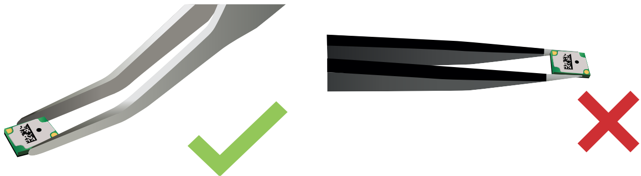
Figure 15: Left: Recommended tweezer type. Right: Not recommended tweezer type
