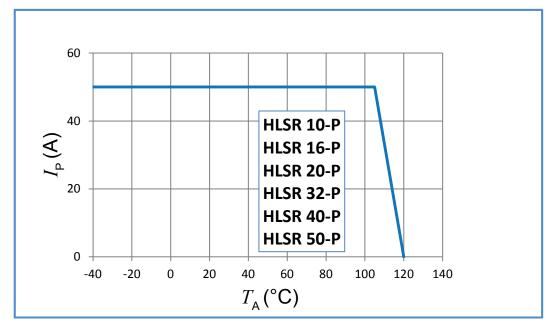
Important notice: whatever the usage and/or application, the transducer jumper temperature shall not go above the maximum ratings of 120 °C as stated in page 2 of this datasheet.
