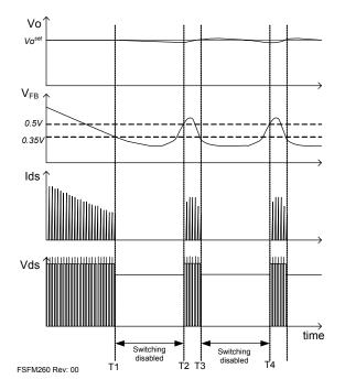
Figure 22. Waveforms of Burst Operation
