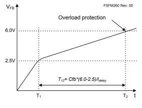
**Figure 20. Overload Protection**
