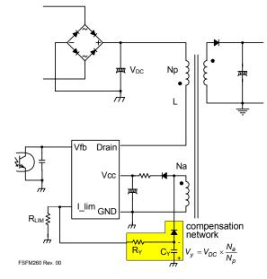
Figure 18. Constant Power Limit Circuit
