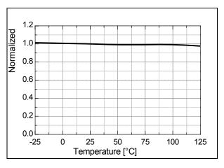
Figure 13. Burst-Mode HIGH Threshold Voltage  $(V_{BURH})$  vs. T<sub>A</sub>
