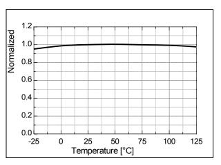
Figure 11. Feedback Source Current (I<sub>FB</sub>) vs. T<sub>A</sub>
