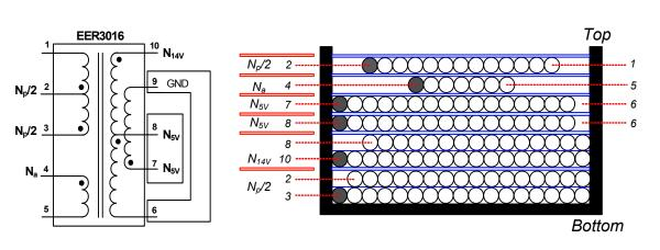
Figure 25. Transformer Schematic Diagram
