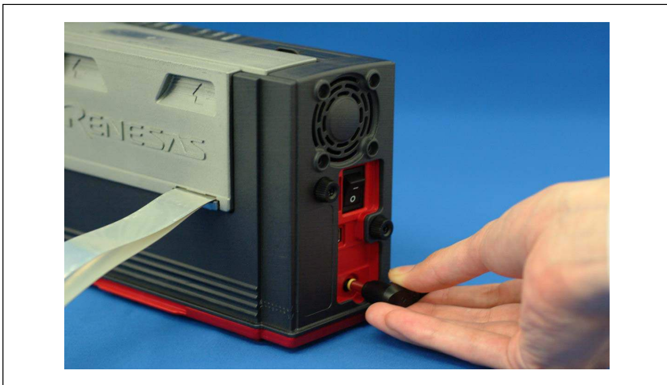
Figure 2.5 Connecting the emulator power supply
