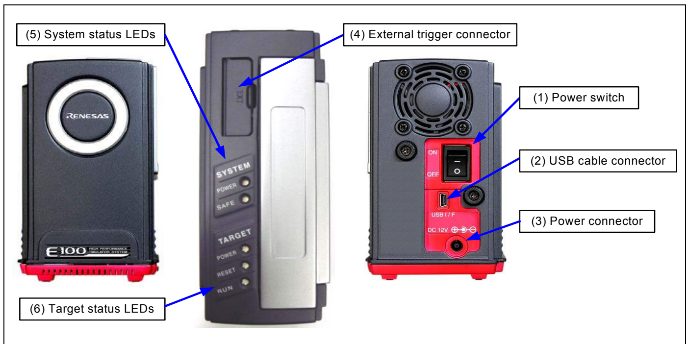
Figure 1.2 Names of each part of the emulator
