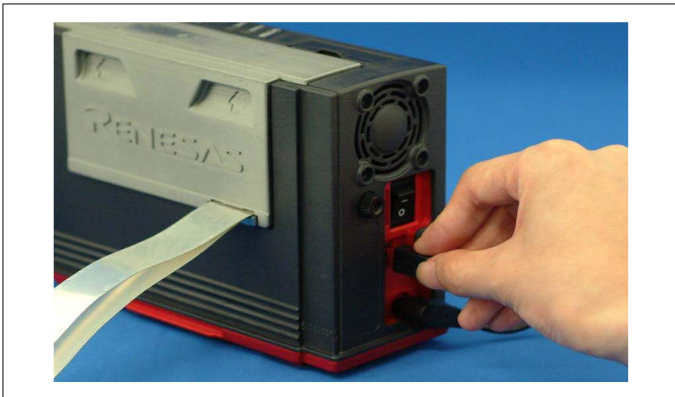
Figure 2.4 Connecting the host machine
