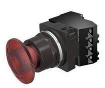
30mm BlackMax, Epoxy Coated Corrosion Resistant Complete Metal Unit Illuminated Twist-to-Release Transformer type, 480V AC LED Lamp Mushroom Head Cap Small 1.79" (45 mm) Plastic Cap, Red 2 Position Maintained, Twist-to-Release with 1 N.O. - 1 N.C. Heavy Duty Contacts, A600/P600 UL Listed, CSA Certified NEMA 1,3,3R,4,4X,12,13 & Automotive Standards
