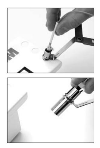
14.2 Remove the connector from the load adapter.
