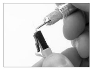
16.3 Pull the fiber straight away from the connector. Pull along the axis of the fiber, not to one side or the other. If the fiber does not pull away, score the fiber again.
