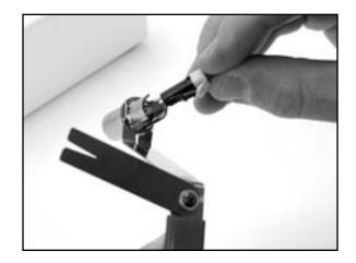
4.5 Place the load adapter, with slot aligned with handle, into an available port in the oven.
