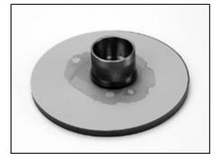
17.11 Polish 10 figure-eight strokes or until bead of adhesive is no longer visible.
