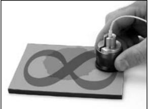
18.10 Leaving the polishing jig assembly positioned on the lapping film, rotate 180 degrees. Perform 3 to 4 additional figure eights.
