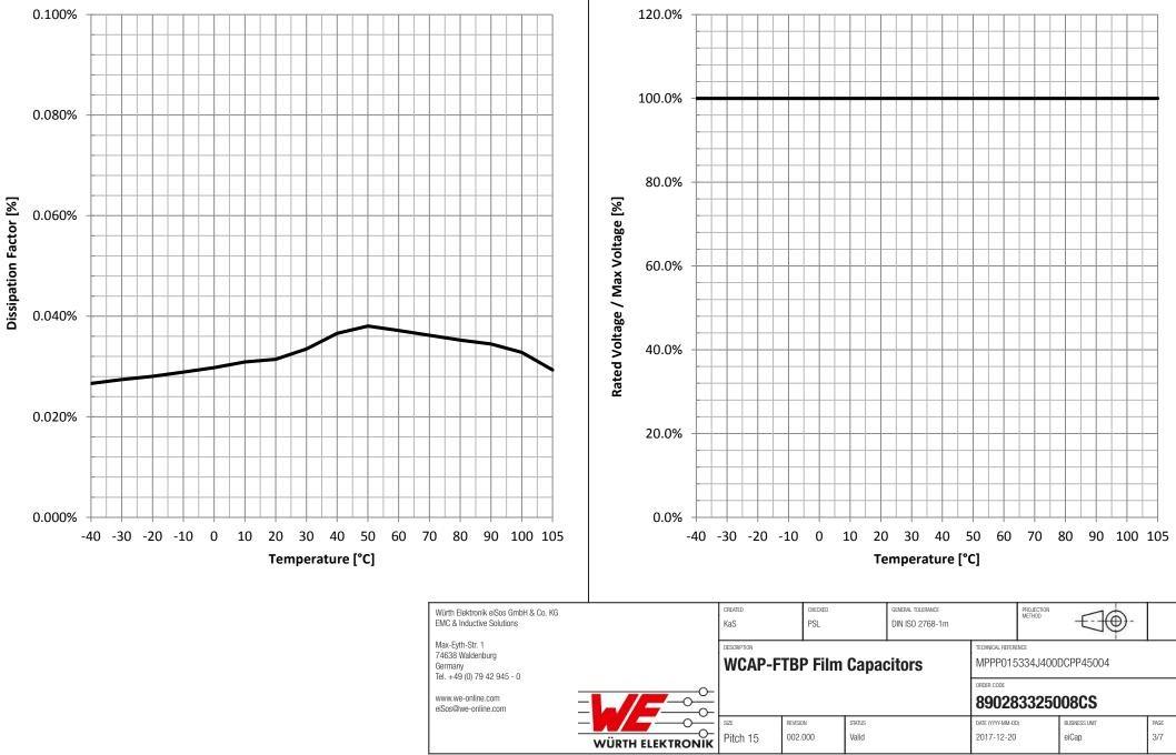
**Rated Voltage vs. Temperature:**
